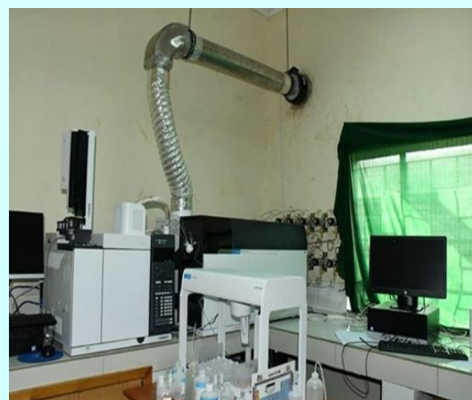
The Gas Chromatography-Inductively Coupled Plasma Mass Spectrophotometer (GC-ICP-MS/MS)
